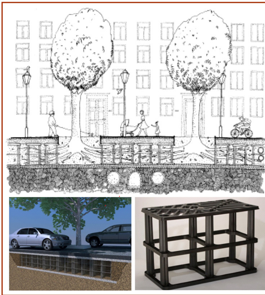
Fig. 9: Cells providing space enough for root growth in streets (Source: Department of Environmental Protection, Capital City of Prague Municipal Office)
