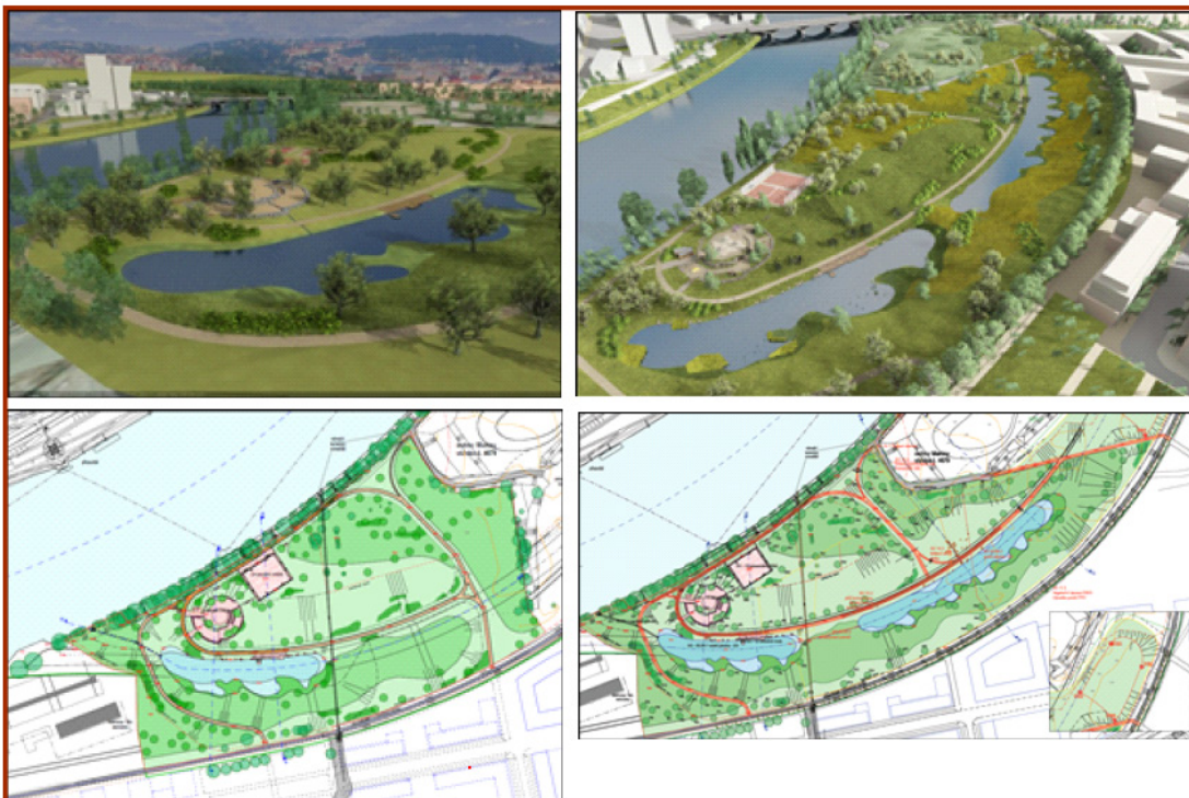
Fig. 17: Flood prevention measures to protect the Capital City of Prague, Stage 000, part 32 Lipenec – Broad-based terrace. The phase of development: a background study has been elaborated (Source: Water Management and Building, pls Prague)
